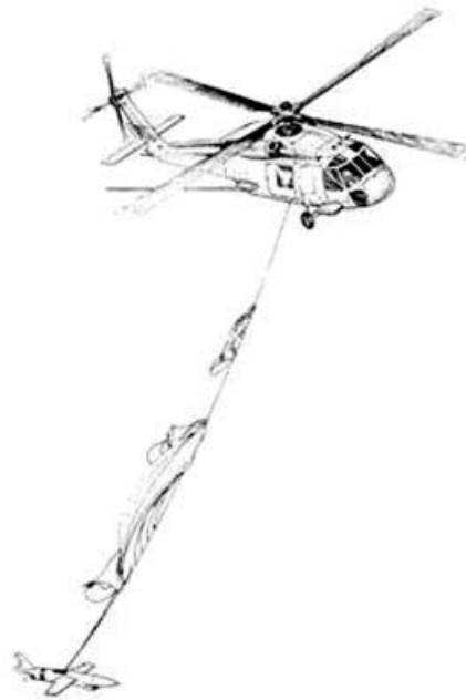
Figure 18.9 Mid-air recovery sequence—snagging (Reproduced by permission of Engineering Arresting Systems Corporation)
