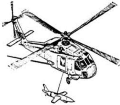
Figure 18.10 Mid-air recovery sequence—recovery (Reproduced by permission of Engineering Arresting Systems Corporation)
