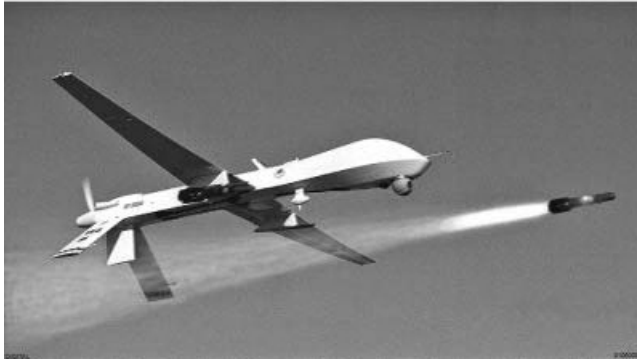
Figure 11.1 Armed Predator, showing missiles on launch rails and optical dome for sensors and laser designator (Reproduced by permission of General Atomics Aeronautical Systems Inc.)
