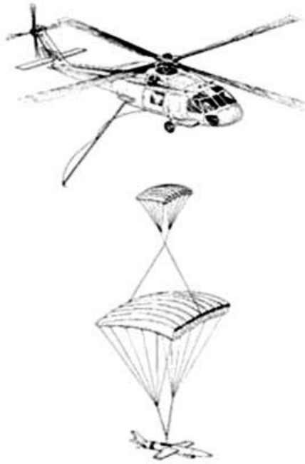
Figure 18.8 Mid-air retrieval (Reproduced by permission of Engineering Arresting Systems Corporation)
